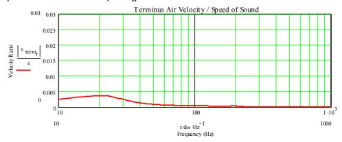
Opposite Bass reflex, a Quarter Wave has stuffing between the driver and the opening. This reduces the displacement (movement of the cone) as seen above. Furthermore, the speed of air in the opening can be controlled, reducing the risk of noise caused by turbulence.
