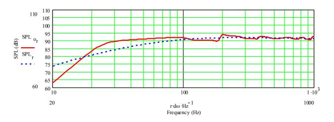
The frequency is dropping perfectly. A flat response is not desirable due to room gain, which has a huge impact on the lowest frequencies. The blue dotted line is SPL in infinitive baffle. The red solid line is the summed SPL from driver and opening.
